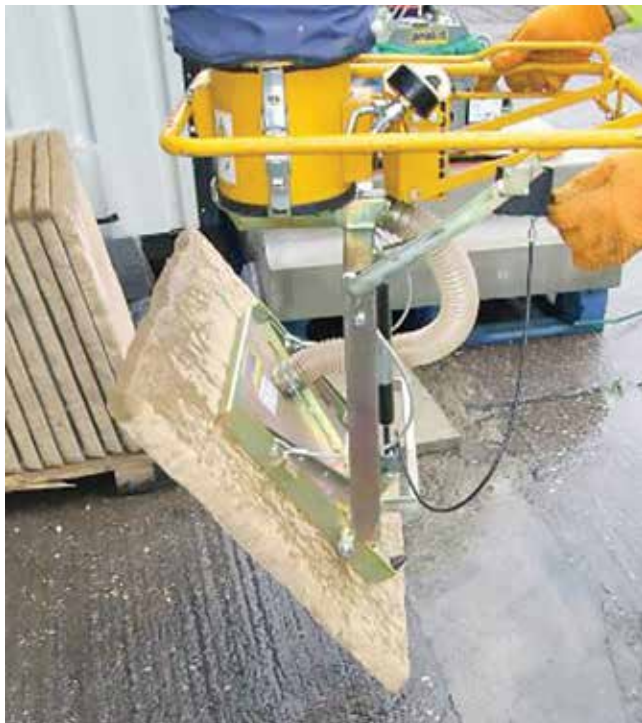
Figures 16 and 17. Vertically stacked paving slabs on a shipping pallet can be lifted, turned to a horizontal position and placed with a vacuum device.
